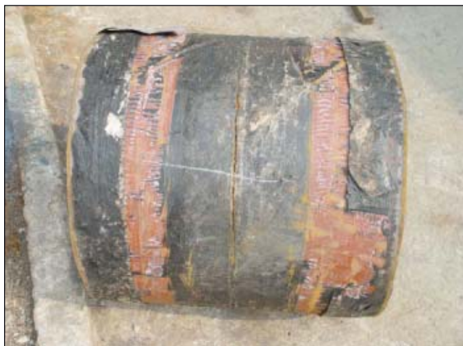
The left end of this cracked pipe section (left photo) was the bent side, with the right end the straight side (Fig. 2). The dark red belt lying close to the inner wall (right photo) shows the weld surface and the original flaw (Fig. 3).
