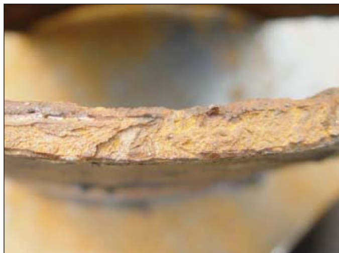
The left end of this cracked pipe section (left photo) was the bent side, with the right end the straight side (Fig. 2). The dark red belt lying close to the inner wall (right photo) shows the weld surface and the original flaw (Fig. 3).
