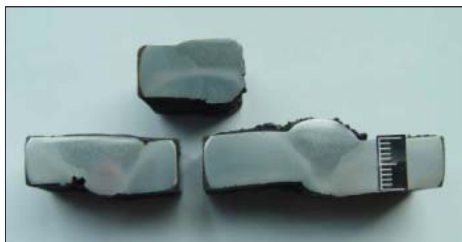
These three specimens show the undercut and offset morphology affecting weld strength where the crack occurred. The upper specimen is from the crack origination. The left specimen, with an undercut of 1.4 mm and 1.4 mm deep crack on its bottom, came from the crack tip. The right specimen, with offsets of 3.5 and 3.0 mm on the inner and outer surfaces, respectively, came from the offset area opposite the crack (Fig. 4).
