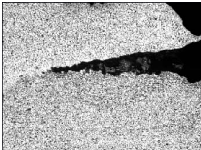
This image (left photo) shows the crack morphology at the undercut bottom of the fracture tip at 25× magnification (Fig. 5). A 100× magnification (right photo) of the fracture tip shows the toe crack (Fig. 6).
